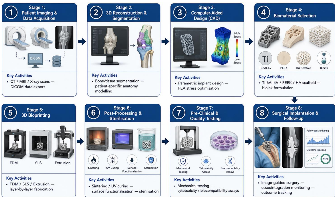
Eight-stage pipeline from patient imaging to post-implantation outcome monitoring. CT = Computed Tomography; MRI = Magnetic Resonance Imaging; FEA = Finite Element Analysis; CAD = Computer-Aided Design.
